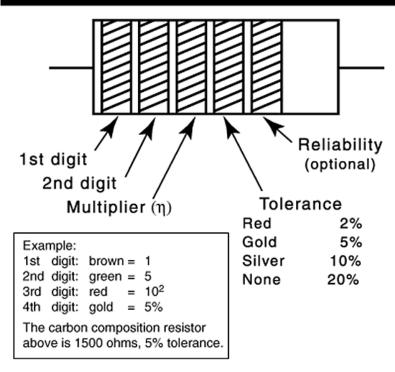
Color-band notation of low-power carbon-composition resistors
